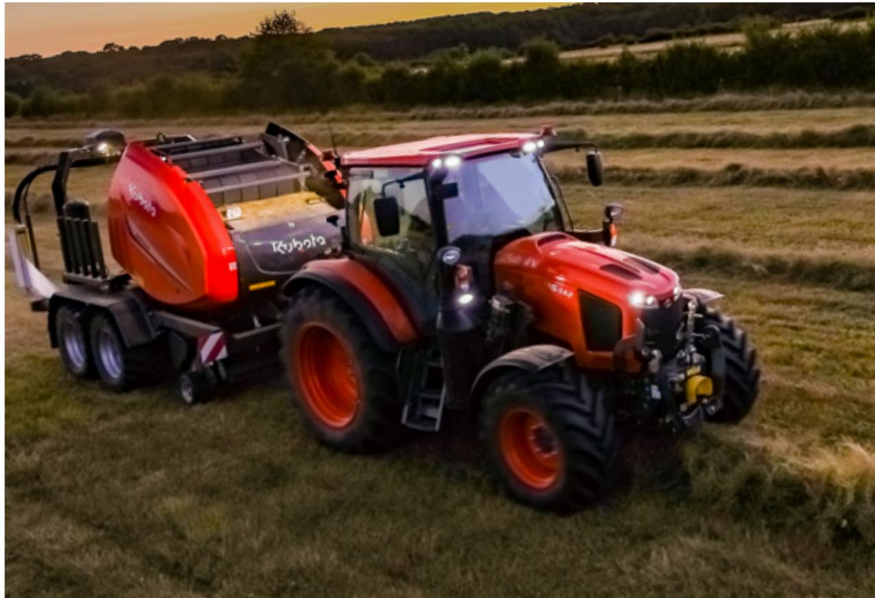
All M6002 Series models are equipped with a CCLS (Closed Centre Load-Sensing) hydraulic pump as standard. This system provides 115 l/min of oil to the hydraulic valves and the front and rear linkages. Three mechanical valves are standard on the M6002, with an additional mechanical valve available as an option. All hydraulic valves are equipped with flow control to optimise the implement work and the tractor also features low-pressure control on the front loader valve.
